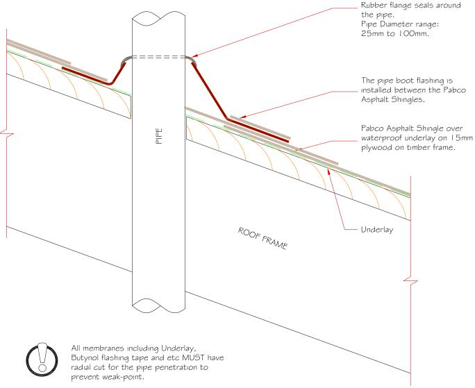
File Name: Scale: Drawn By: 2.81 - Penetation Detail - Pipe.dwg 1:2 @ A4 I.M 28th January 2013 Sheet: Penetration Junction Detail - Pipe 16
